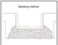
edge of the channel to the string line. Pull bedding concrete around lower anchoring ribs. After concrete bedding sets, sidewall sections can be installed, if necessary, and the final pour can be made.
